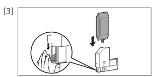
Lower the lock lever on the High capacity ink pack adapter and insert the ink bag.
