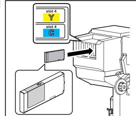
Re-insert the ink cartridges into lnk cartridge slots.
