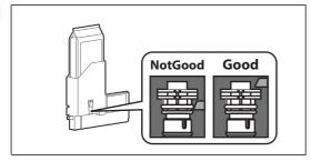
Confirm ink bag is fully seated by checking the lock mechanism is at the top of the ink delivery neck through the observation window, see proper placement in illustration left. [5]
