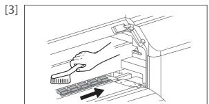
Brush off dusts on the pressurizing rollers with a soft brush.
