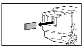
Remove ink cartridges from Ink cartridge slots.
