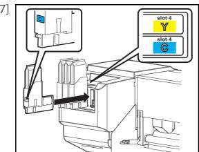
Re-insert the High capacity ink pack adapters into Ink cartridge slots.
