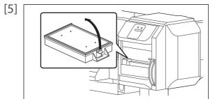
Pull the tab up of the absorption material for the flushing box, and release the hook.
