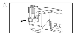
Remove High capacity ink pack adapters from the ink cartridge slots.
