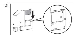
Slide the smart chip card into the tab on the High capacity ink pack adapter to install it.
