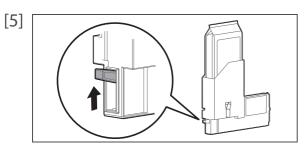
Confirm that the lock lever on the High capacity ink pack adapter is in its original position.
