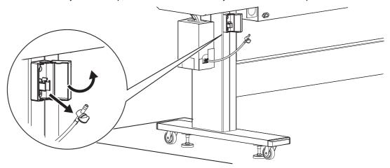
[5] Put the tip of the two-way valve in the empty container and open the two-way valve to drain waste ink from the waste ink tank.
