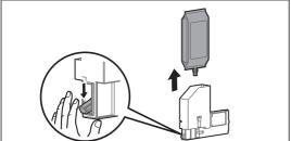
Lower the lock lever on the High capacity ink pack adapter and detach the empty ink bag.
