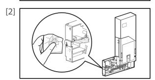
Using the paper towel provided with the printer to wipe off the ink attached to the insertion point for High capacity ink pack adapters.
