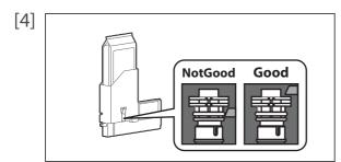
Confirm that the ink bag is inserted all the way and is locked.
