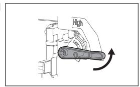
Change the head height by moving Head height adjustment lever (orange).
