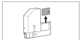
Remove the S/C card from the High capacity ink pack adapter.
