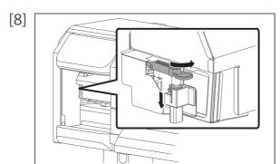
Press the tab of Cutter lightly, return cutter cap to its initial position.
