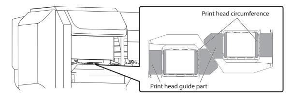
[2] Use the cleaning stick to remove the ink and dust on the bottom of the carriage.
